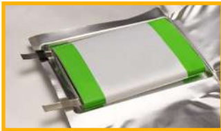
Packaging of separator electrode assembly into pouch cell laminate
