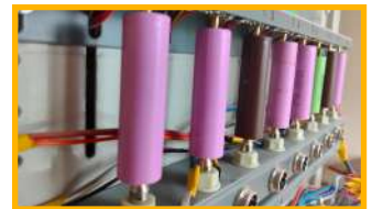
Long term cycle life testing on cylindrical cells
