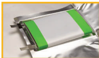
Packaging of separator electrode assembly into pouch cell laminate
