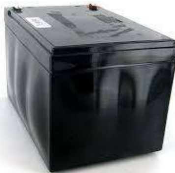
Figure 56 Image of a bulged lead acid battery
