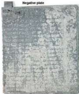
Figure 14 A hard sulfated negative plate
